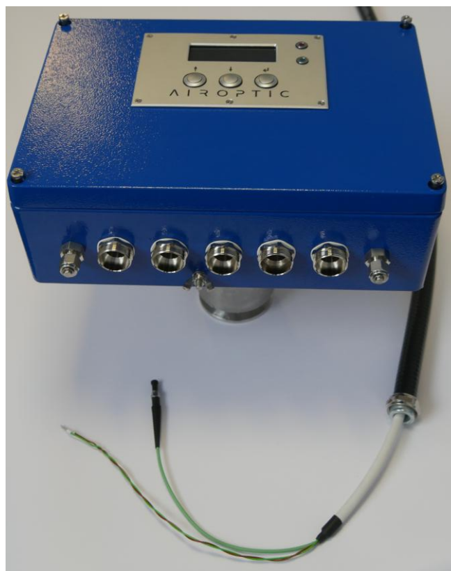
Figure 259. Inserting hybrid loop cable into transmitter
