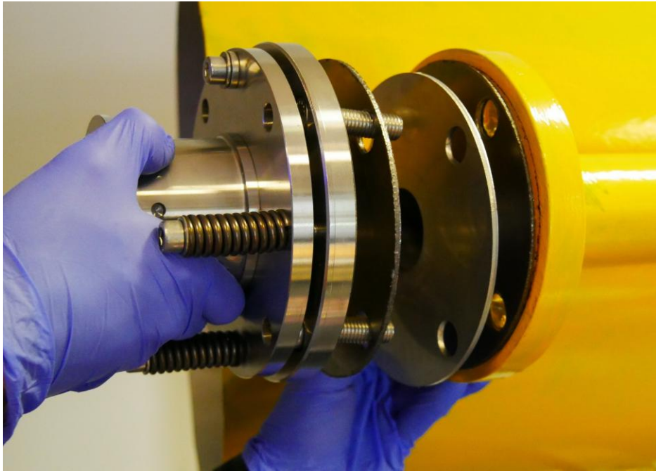
Figure 18. ETC - mounting flange on the process flange.
