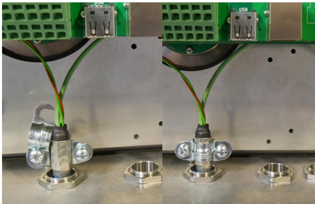
Figure 77. Fiber cable connector grounding (stainless steel glands version).
