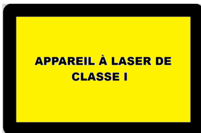
Figure 237. Warning label - Internal invisible IR laser is a Class I product – french version.
