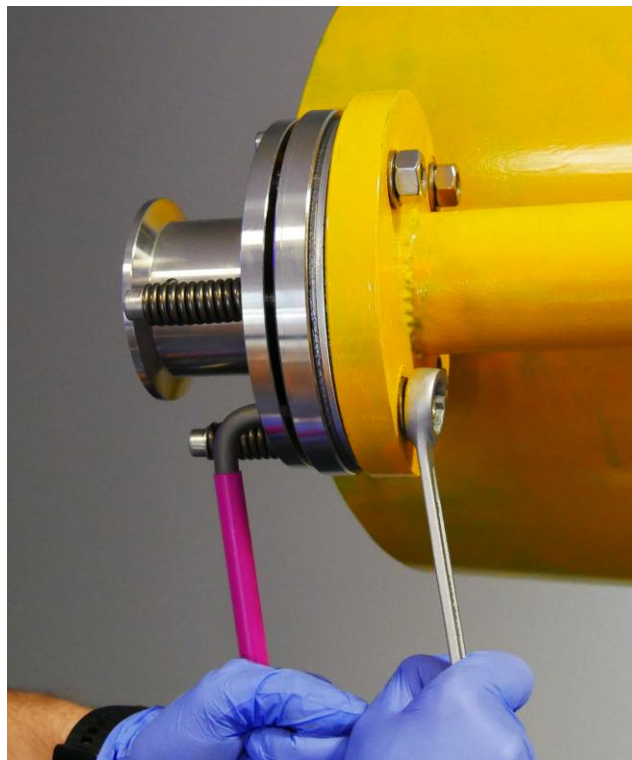
Figure 19. ETC - Nuts mounting.
