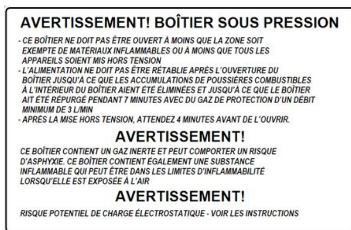
Figure 233. Warning label for analyzer enclosures lids – french version.
