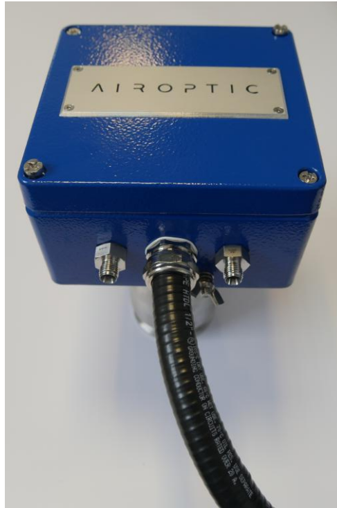
Figure 256. Fastening the conduit gland
