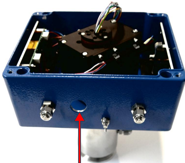
2. Insert the conduit laser cable through the hole on the transmitter unit shown in the figure below
