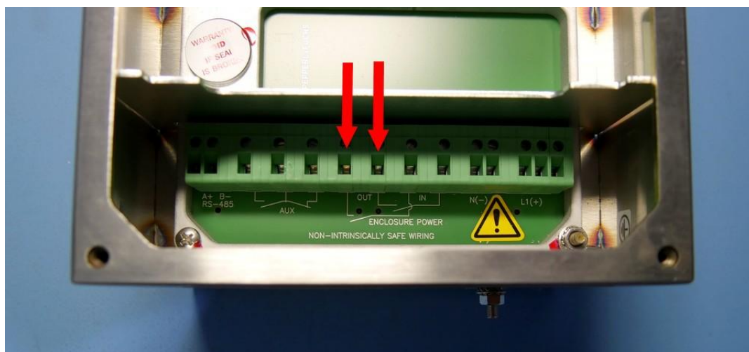
Figure 212. Supply connectors for powering the analyzer.
