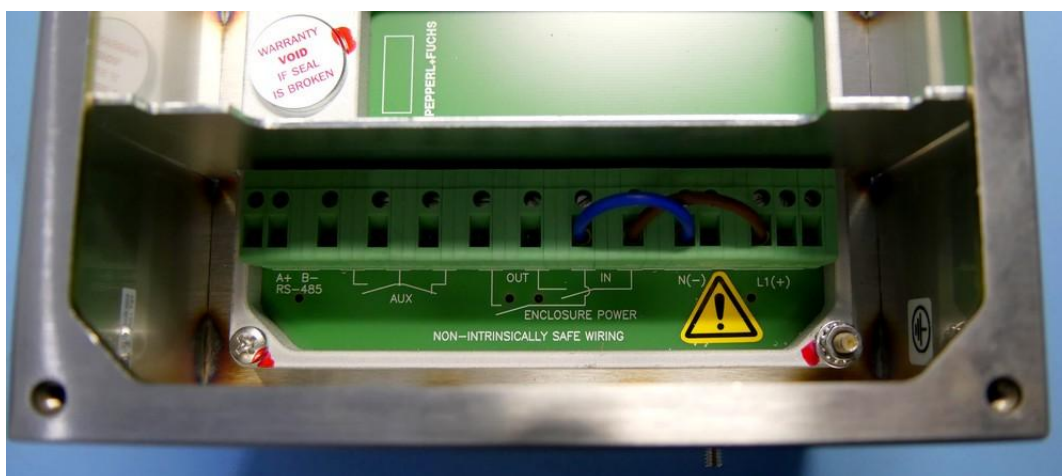
Figure 213. Jumpers placement for powering the main supply switch in purge controller.
