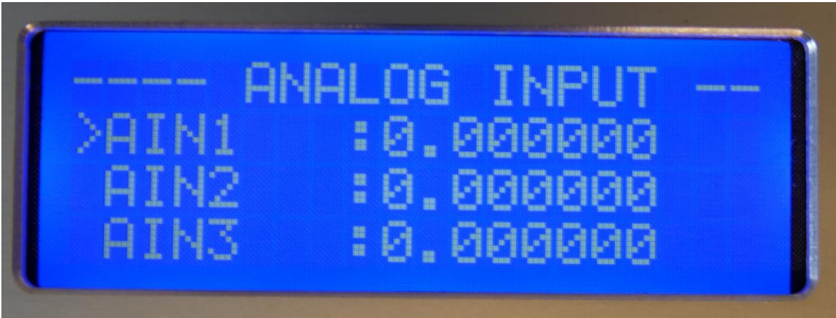
Figure 49. Front panel display – analog input AIN1-3.
