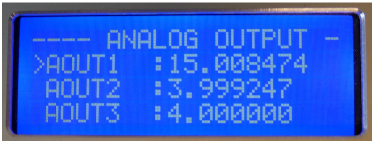
Figure 51. Front panel display – analog output AOUT1-3.
